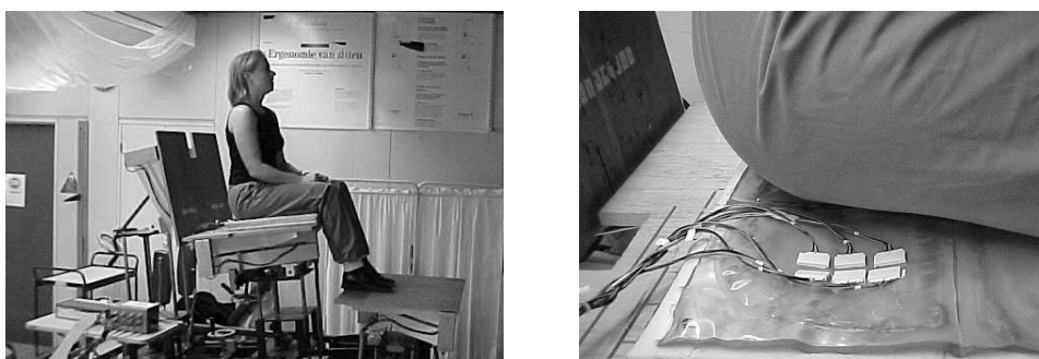
Figure 1. [Left] The measurement of shear stress on the right ischial tuberosity of a subject while sitting on the LiquiCell cushion in the backward tilted situation. [Right] Detail of the six shear sensors that are placed underneath the right ischial tuberosity (subject has lifted her buttocks for the picture).
